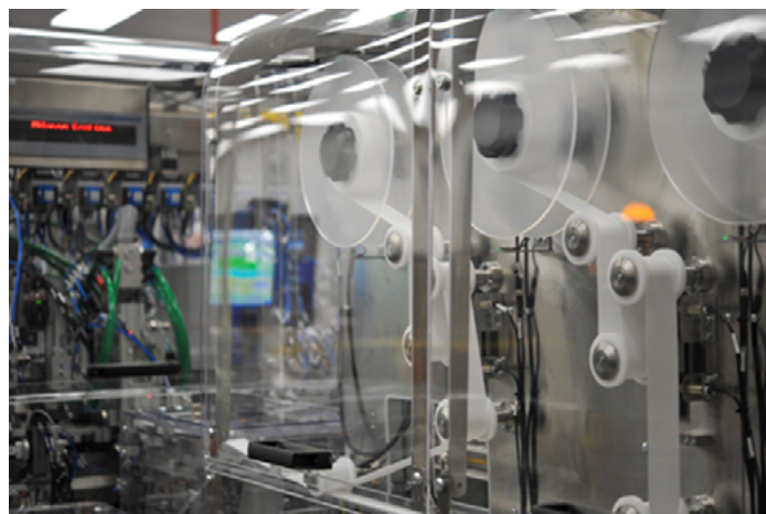
Reel-to-reel assembly and lamination of multi-layer test strips support high-speed manufacturing for large-scale medical testing programs. (Photo courtesy of Web Industries.)
